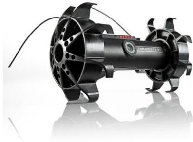
Once deployed, the micro-robot can be directed by the operator to quietly move through a structure and transmit video and audio reconnaissance to the handheld Operator Control Unit II (OCU II). These stealth capabilities can be utilized to locate armed subjects, confirm the presence of hostages or innocent civilians, listen in on conversations, and reveal the layout of rooms – information that can save lives and increase the success of high-risk operations.
